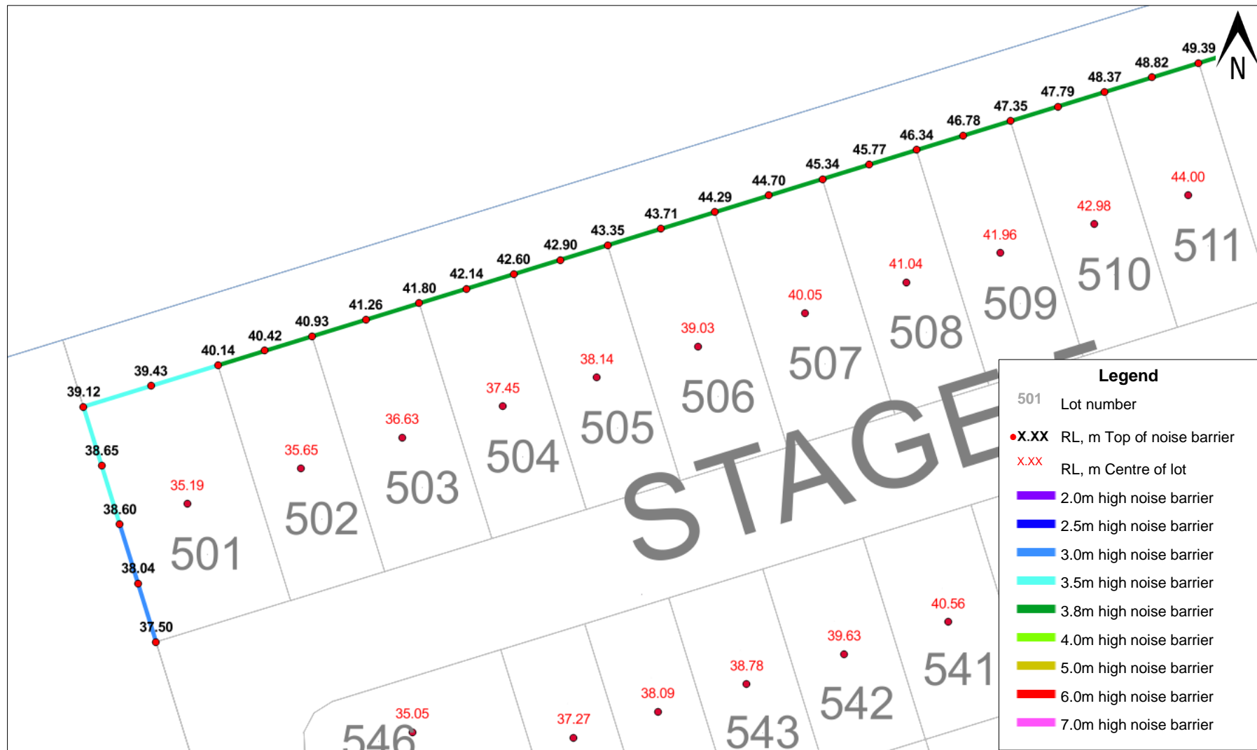
Figure 4.8 Noise barrier alignment – Scenario 2 – Detail 1
